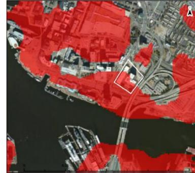
**Airborne LiDAR High Resolution Elevation Map** – This illustrates detailed elevation information for the extent of the site. It provides a visualization of low lying areas and helps give context to the results of the CRRA, FIRST Score™ and SLOSH models, assisting with evaluation, prioritization, and decision-making.
